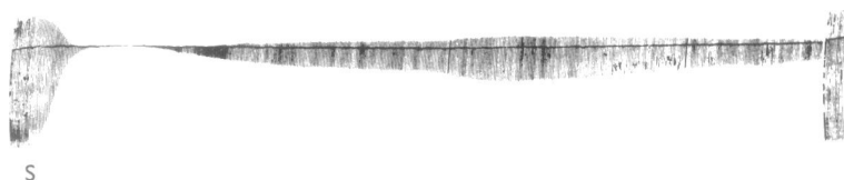
FIG. 4. Biphasic response of an isolated diaphragm preparation immersed in normal Krebs solution in the continuing presence of suxamethonium, 5.0 \times 10^{-6} g/ml (S). Contact time 75 min.
